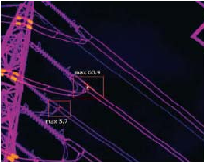
Image taken with 640x480 pixel resolution and <math><45\text{mK}</math> thermal sensitivity. Notice how the hot spot now is clearly visible and that the increased number of pixels will result in an even more accurate temperature reading in the hot spot. It is now clear that there is a problem in the power line.
