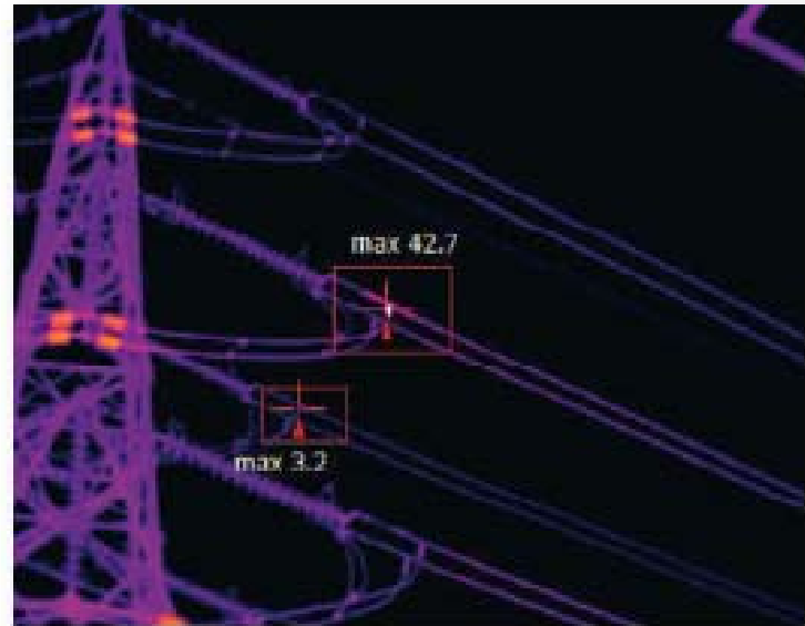
Image taken with 320x240 pixel resolution and 50mK thermal sensitivity. Please note how the increased number of pixels will result in a more accurate temperature reading in the hot spot.
