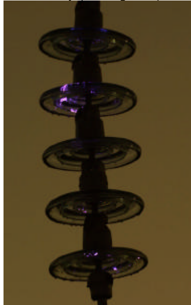
Figure 5: Non-Uniformly Polluted/ Wetted String (top side clean and dry)
