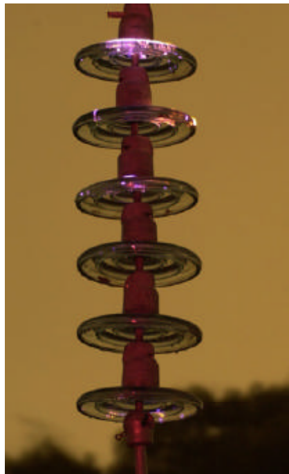
Figure 3: Insulator String Uniformly Polluted/Wetted
